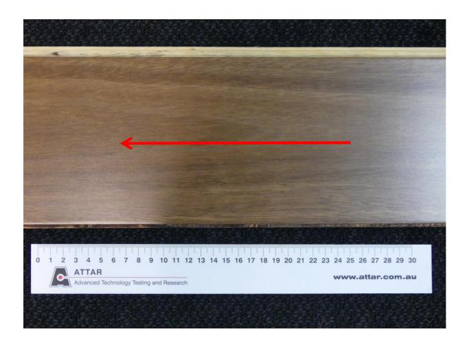
Figure 1: Eng Aust. Species semi-gloss plank Arrow indicates direction of testing
