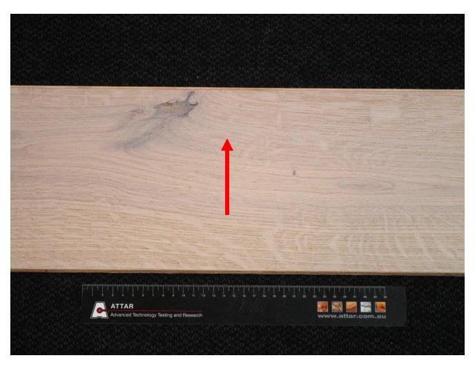
**Figure 1:** De Marque Engineered Oak 120, 190, 240 & 300 mm stair tread and nosing. Arrow indicates direction of testing.
